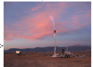
Gas flare measuring methane at the Templeton Gap Landfill, Colorado
