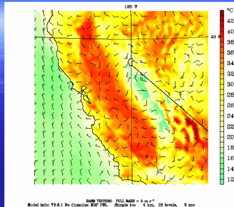
**Simulated temperature and winds at 1600 PST on July 31st (left) and August 1st (right) 2000, at  $\sigma = 0.999$ , for Central California.**
