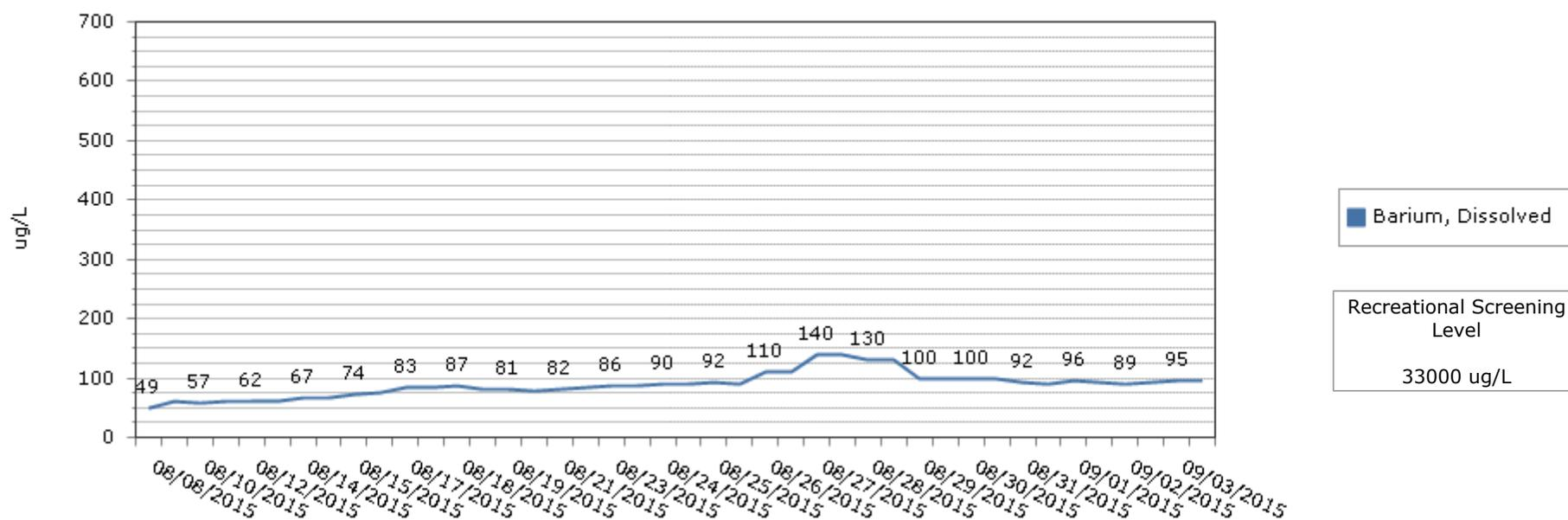
For samples with metal concentrations that were too low to detect, EPA plotted the Method Detection Level (MDL) value onto the trend graph.
