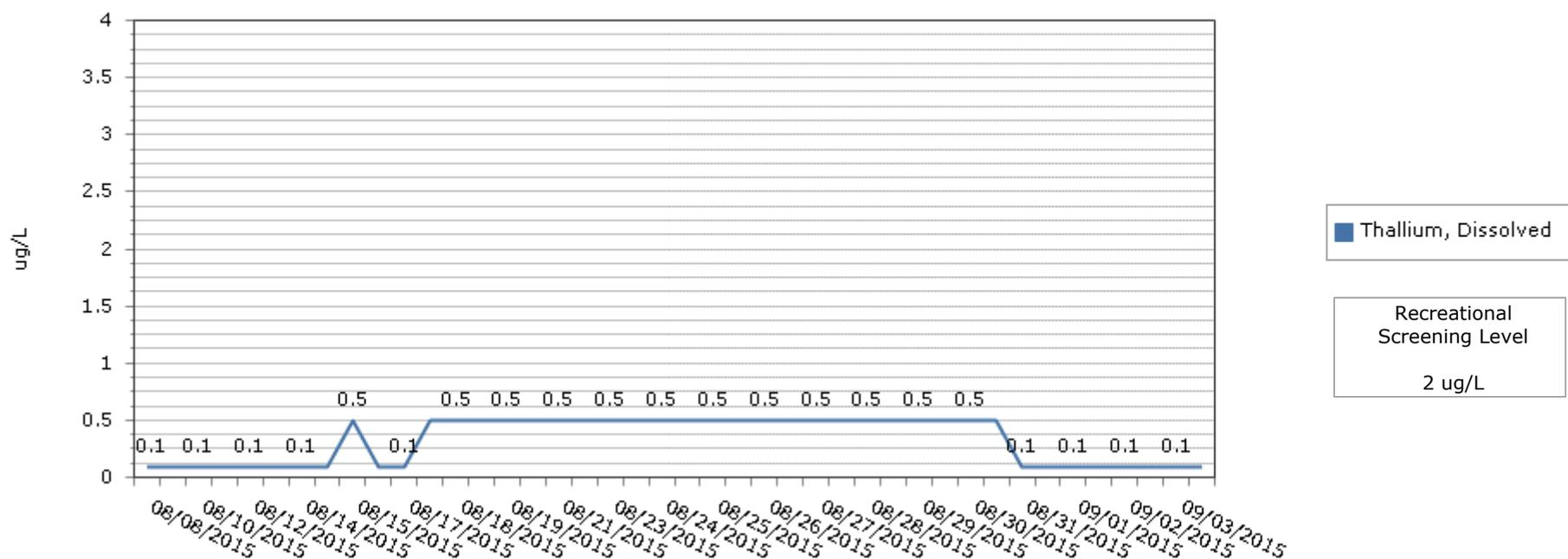
For samples with metal concentrations that were too low to detect, EPA plotted the Method Detection Level (MDL) value onto the trend graph.
