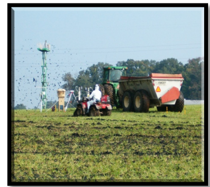
Conducting Bioaerosol Sampling Behind Biosolids Applicator
