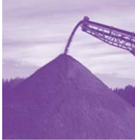
Crushed asphalt on conveyer belt.
