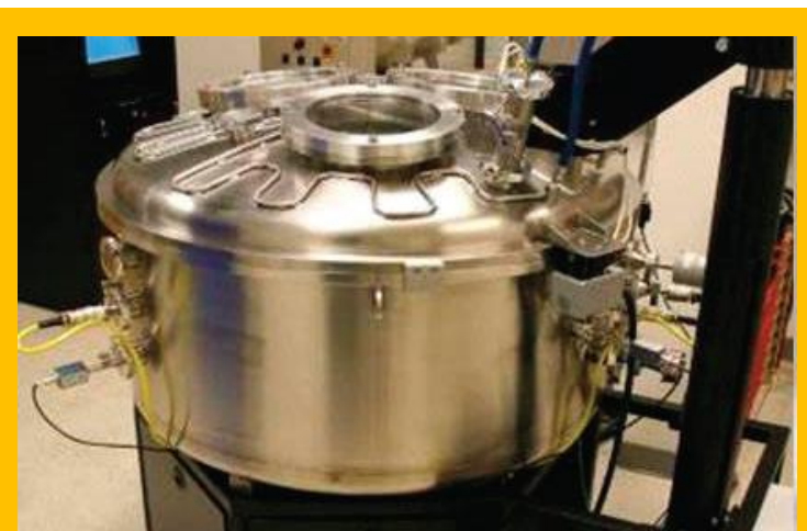
Mold coating takes place in a fully automated chamber (above) without exposing workers to toxic chemicals (below).
