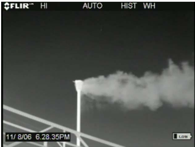
Exhibit 1 Infrared Camera Display of Gas Plume Invisible to the Eye
