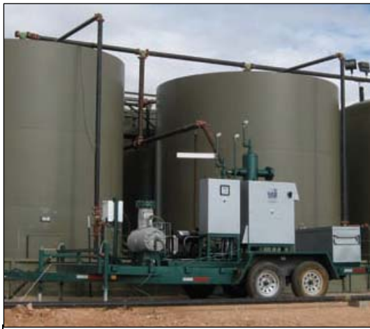
Exhibit 2. Skid-mounted scroll VRU
