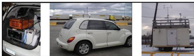
(L) air monitoring vehicle used in study. (R) the stationary air monitor.
